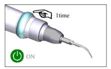
To switch the power on press the ring switch. At the same time, the STATUS indicator will blink several times and light up in MINT color,
