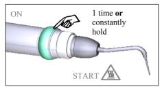
Press the ring switch briefly **OR** press and hold to switch the heating mode on During 1,0 - 1,6 sec. the thermoplugger is heating to the set working temperature. The STATUS indicator on the handpiece **blinks ORANGE**
