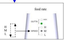
The parameter is changed cyclically. A white "SPEED" indicator lights up next to the name of the selected feed rate.
