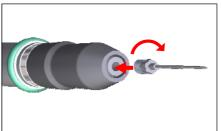
A) Screw the injector needle into the thread hole in the heater by turning needle the clockwise
