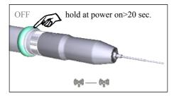
Press and hold the ring switch at switching the power on. After 3 cycles of the audio signals with different intensity and 1 single audio signal (wait for 20 sec.) STATUS
