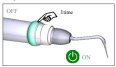
To switch the power on press the ring switch.
