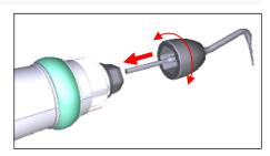
Install the thermoplugger into the handpiece socket.
