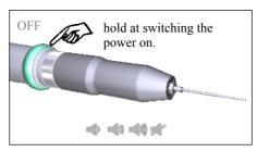
To choose the required volume level stop pressing the ring switch.
