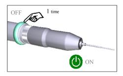
To switch the power on press the ring switch.
