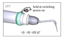
To select the required volume level hold the ring switch when switching the power on. Within ~10 sec. volume levels change one another cyclically.
