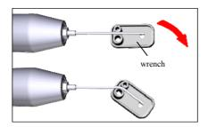
If necessary, use the multifunctional wrench to give the injector needle a smooth curvature so that the needle can extend about 5 mm beyond the working length of the canal.
