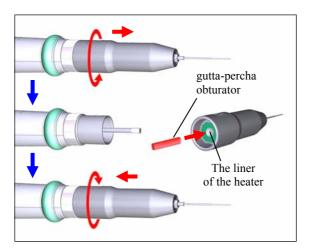
Never use force if the heater fails to be fixed in the handpiece control unit or, conversely, you cannot disconnect it from the control unit. If the problem takes place see section 9 "Troubleshooting"
